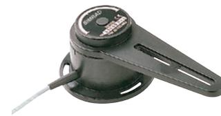
Rudder feedback units are small sensors that measure and report rudder position, enabling precise rudder control for smooth and accurate steering. On smaller boats, Virtual Rudder Feedback (VRF) eliminates the need to install a physical sensor by using a software-based approach to calculate rudder position.
